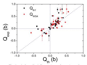
Fig. 3. (color online) Comparisons of experimental NQMs with the results of the shell model calculations and this paper. The theoretical values of  $Q_{\rm th1}$  (black squares) are derived from the pf-shell model calculations [28], and the theoretical values of  $Q_{\rm WS4}$  (red circles) are the results of this paper with deformation parameters derived from mass model WS4. The experimental data are taken from Ref. [24].
