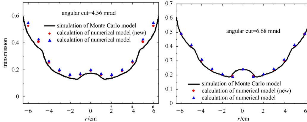
Fig. 3. (color online) Comparison of the Monte Carlo model and numerical model results for the FTO.
