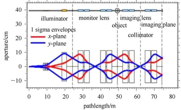
Fig. 1. (color online) The proton radiography setup used for the Monte Carlo simulation.
