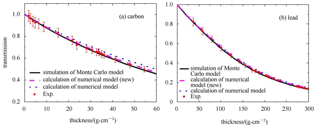
Fig. 2. (color online) Comparison of Monte Carlo simulation and numerical model calculation results with experimental data for carbon (a) and lead (b).
