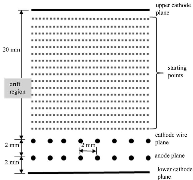
Fig. 1. Structure of the MWPC.
