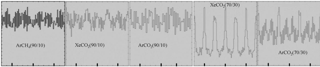
Fig. 7. Best UIR spectrum of the detector using different working gases with drift region depth of 20 mm; the markers on the  $x$ -axis represent the positions of the anode wires.
