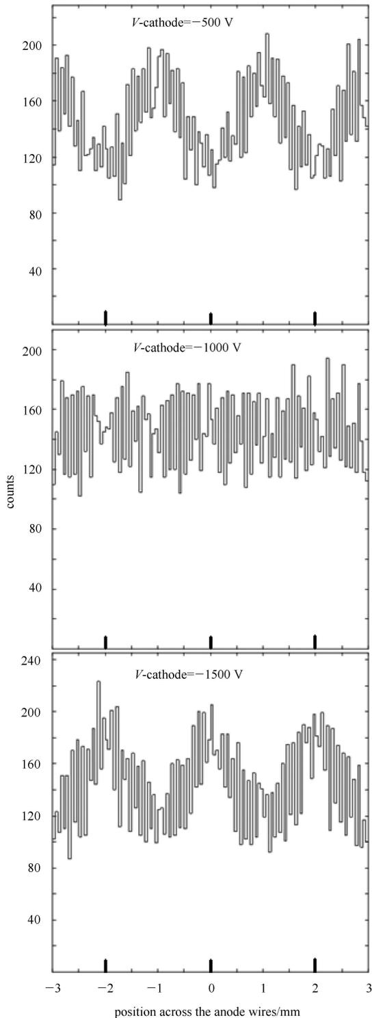
Fig. 6. UIR of the detector under different cathode voltages. The anode wires are located at 0,  $\pm 2$  mm.
