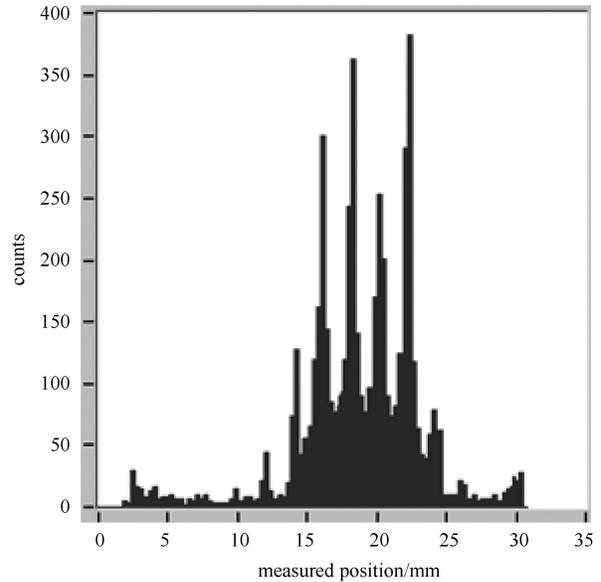
Fig. 5. Measured position response of the detector for a collimated X-ray beam.
