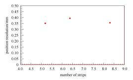
Fig. 14. The Gaussian width (defined in formula 5) relative to the number of strips per cluster used for position calculation. The *x*-axis is the number of strips per cluster used for position calculation.
