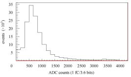
Fig. 6. Distribution of signal magnitudes of the peak signal in each cluster. The *x*-axis is the digitized charge collected.
