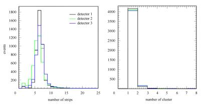
Fig. 9. (color online)For pTGC- I : (Left) Distribution of cluster sizes (number of strips in a single cluster). (Right) Number of clusters in a single chamber per triggered event.
