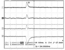
Fig. 4. The observed signals on the wires and several copper strips, induced by the same incident cosmic ray. The signal on the wire is negative, while the signals on the strips are positive.
