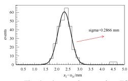
Fig. 12. The distribution of  $x_2-x_{2c}$  for pTGC-II. The corresponding position resolution of the chamber is  $\sigma = \frac{w}{\sqrt{2\pi M^2}} = \frac{286 \ \mu\text{m}}{1.22} = 233 \ \mu\text{m}.$
