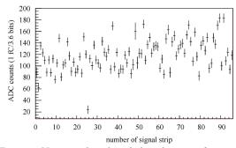
Fig. 5. Noise and pedestal distribution of 96 signal strips in one chamber (the *x*-axis is the signal strip number, the vertical coordinate is the pedestal value and the error bars represent the noise of that channel.)
