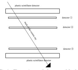
Fig. 3. The cosmic muon hodoscope used for the chamber testing. Plastic scintillator detectors are used for the trigger, and three identical pTGC chambers are placed in parallel between the two scintillator detectors.
