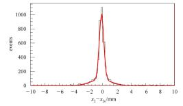
Fig. 11. The distribution of  $x_2-x_{2c}$  for pTGC-I. The corresponding position resolution of the chamber is  $\sigma = \frac{w}{\sqrt{1+k^2}} = \frac{500 \ \mu\text{m}}{1.22} = 409 \ \mu\text{m}.$
