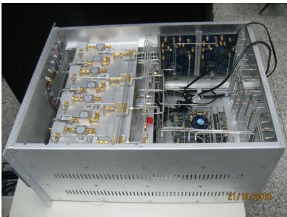
Fig. 3. The layers of the LLRF control box.
