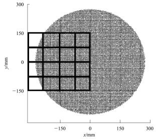
Fig. 4. The position distribution of scattered <sup>12</sup>C on the MWPC and the CsI detectors. The circle and the square correspond to the distribution on the MWPC and the CsI detectors, respectively.
