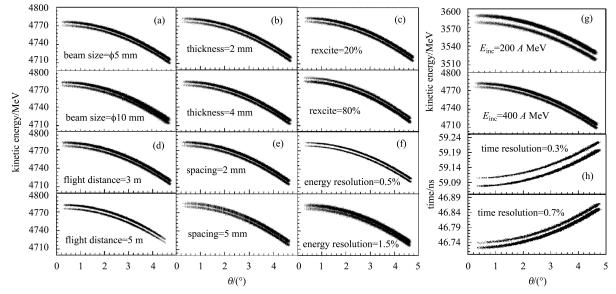
Fig. 3. The relation between scattering angles (from 0° to 5°) and scattering kinetic energy with different variable parameters which correspond to (a) beam size, (b) target thickness, (c) excited ratio of the excited state with 4.4 MeV, (d) flight distance, (e) wire spacing of the MWPC, (f) energy resolution of the CsI detectors, (g) incident kinetic energy, besides (h) for the relation between scattering angles and TOF with time resolution of the plastic scintillators.
