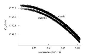
Fig. 2. Relation between the scattering angles  $\theta$  and the actual detected kinetic energy  $E_{obs}$ .
