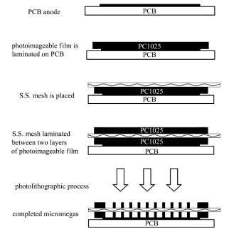
Fig. 2. The process of bulk micromegas fabrication.
