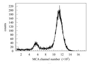
Fig. 4. The spectrum of <sup>55</sup>Fe 5.9 keV X-ray has an energy resolution of full energy peak which is 16% (FWHM). (95% argon, 5% isobutane).
