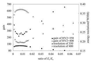
Fig. 6. The gain and energy resolution versus the ratio of  $E_{\rm c}$  to  $E_{\rm a}$ .
