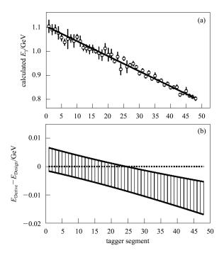
Fig. 5. Calibration of the photon tagging system. The errors showing in the (a) are the fitting error for each segment, the curve is a linear fitting; the (b) figure gives the propagation of the fitting for derived  $E_{\gamma}$  respecting to the designed  $E_{\gamma}$ .
