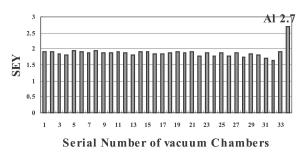
Fig. 4. Measured SEY of TiN-coated chambers.
