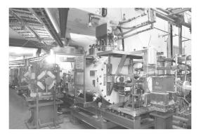
Fig. 3. A superconducting cavity in installation.
