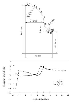
Fig. 2. Segment location and sensitivity of the frequency shift by errors in R and Z.
