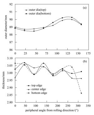
Fig. 4. Peripheral distributions of the outer diameter (a) and wall thickness (b) at the top and bottom edges of the niobium beam pipe after rolling.
