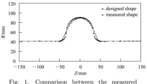
shape and the designed shape for the niobium cavity.
