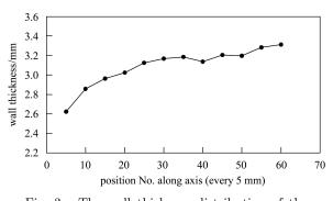
Fig. 3. The wall thickness distribution of the niobium half-cell along the axis direction after deep drawing.
