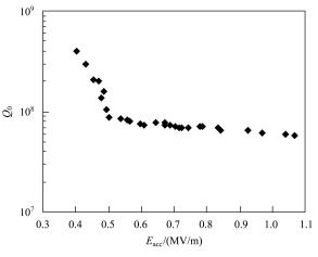
Fig. 5.  $Q_0$  versus accelerating field curve at 4.2 K for the niobium cavity just after ultrasonic rinsing.
