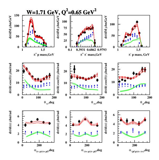
Fig. 2. Resonant (bars) and non-resonant (lines) contributions to the charged double pion differential cross sections at W = 1.71 GeV and  $Q^2 = 0.65$  GeV<sup>2</sup>. The full JM calculation are shown by solid red lines. The experimental data are from <sup>[2]</sup>.
