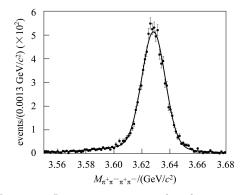
Fig. 3. Invariant mass distribution of  $\pi^+\pi^-\pi^+\pi^-$  from MC simulation of  $\psi' \rightarrow \gamma \eta'_c$ ,  $\eta'_c \rightarrow \pi^+\pi^-\pi^+\pi^-$  based on BOSS. The smooth line is the best fit to the mass distribution using a double-Gaussian.
