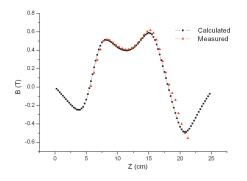
Fig. 2. The measured and calculated axile magnetic field.
