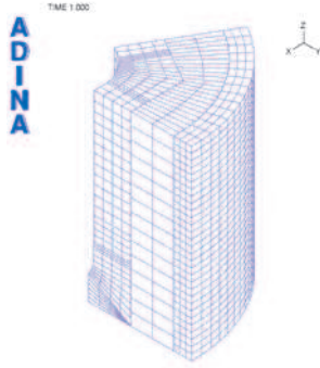
Fig. 3. FE-model of the sextupole magnet structure.
