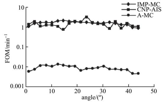
Fig. 16. FOM curves of neutron flux at pressure vessel 1/4 peak axial location ( $E > 1.0 \text{ MeV}$ ).
