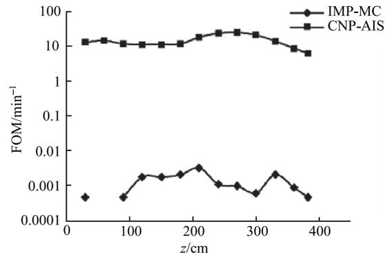
Fig. 9. FOM curves of neutron flux axial distribution in biological shield wall.
