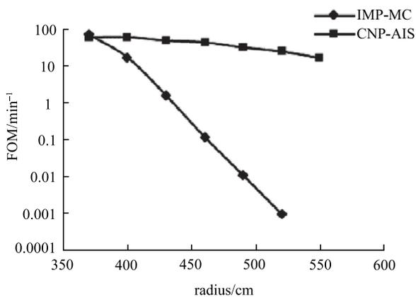
Fig. 5. FOM curves of neutron flux radial distribution in biological shield wall.
