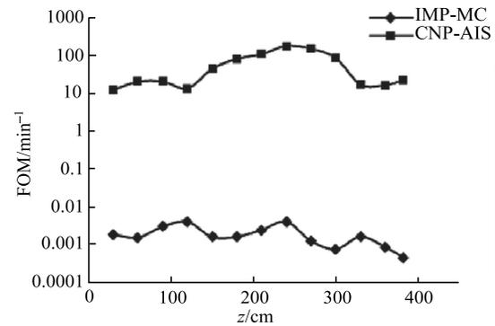
Fig. 10. FOM curves of photon flux axial distribution in biological shield wall.
