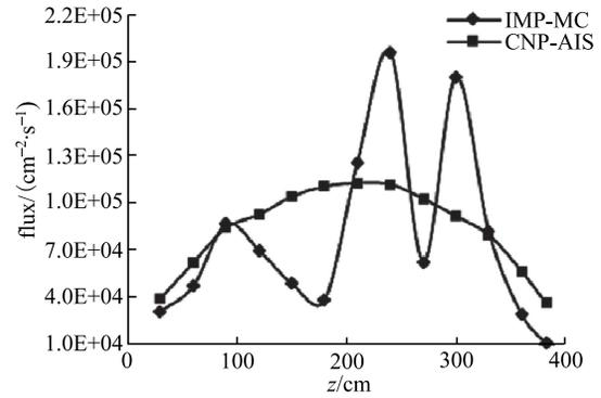
Fig. 8. Photon flux axial distribution in biological shield wall.
