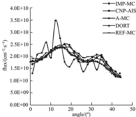
Fig. 15. Neutron flux at pressure vessel 1/4 peak axial location ( $E > 1.0 \text{ MeV}$ ).
