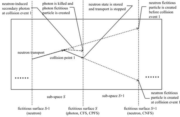
Fig. 3. Particle transport in the CNP-AIS method.
