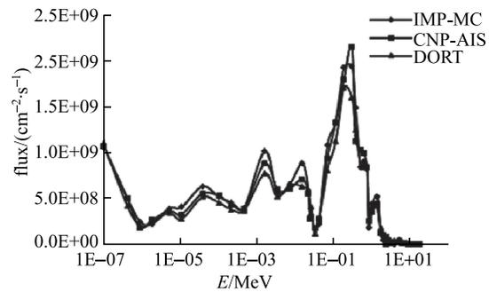
Fig. 13. Neutron flux spectrum at capsule location.
