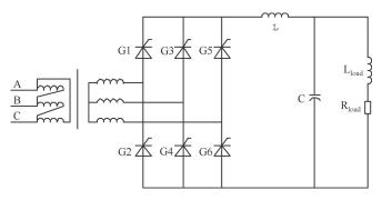
Fig. 7. Schematic of MPS prototype.
