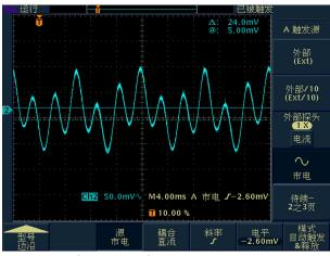
Fig. 10. (color online) Waveform of current ripple with MPS working at 24 A.
