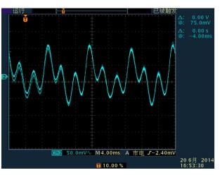
Fig. 12. (color online) Waveform of current ripple with MPS working at 40 A.
