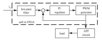
Fig. 8. APF control loop in FPGA.
