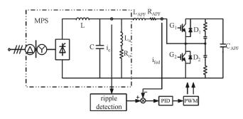
Fig. 5. Schematic of APF control loop.
