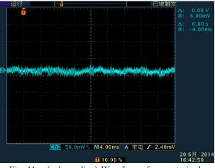
Fig. 11. (color online) Waveform of current ripple with APF connected, with MPS working at 24 A.
