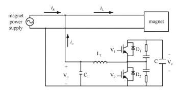
Fig. 2. Schematic of new APF topology.
