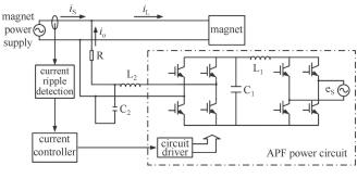
Fig. 1. Principle diagram of APF.
