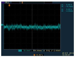
Fig. 13. (color online) Waveform of current ripple with APF connected, with MPS working at 40 A.
