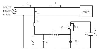
Fig. 4. APF working as a Buck circuit.
