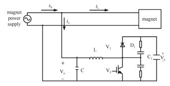
Fig. 3. APF working as a Boost circuit.
