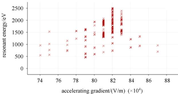
Fig. 5. (color online) MP resonant energy vs. accelerating gradient around the beam pipe.
