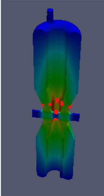
Fig. 4. (color online) MP location around the beam pipe.
