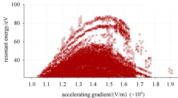
Fig. 7. (color online) MP activity resonant energy vs. accelerating gradient in the rinse port.
