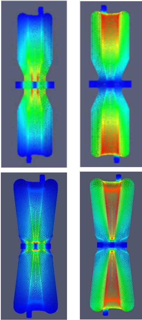
Fig. 2. (color online) The electric (left) and magnetic (right) field distributions of the HWR cavities (top: HWR-010; bottom: HWR-015).
