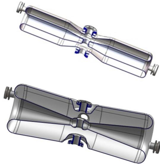
Fig. 1. (color online) Schematics of the HWR cavities (top: cylinder type HWR-010; bottom: taper type HWR-015).
