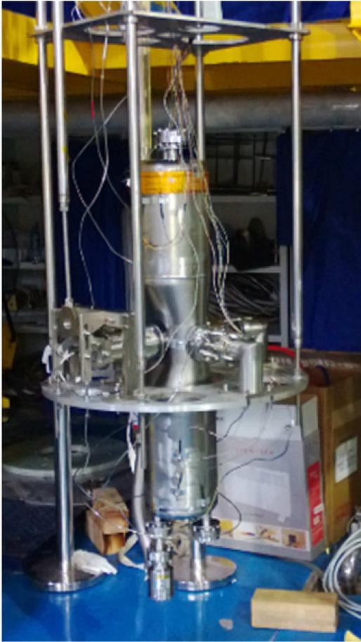
Fig. 8. (color online) HWR-010 cavity installed in vertical test stand.
