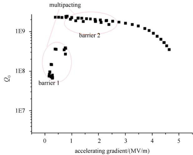
Fig. 9. (color online) Vertical test quality factor vs. accelerating gradient for HWR-010.
