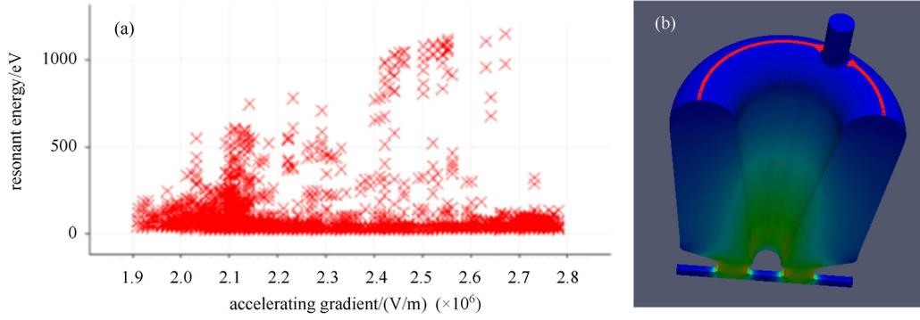
Fig. 11. (color online) Resonant energy vs. accelerating gradient (a) and relevant MP location on the shorting plate (b).
