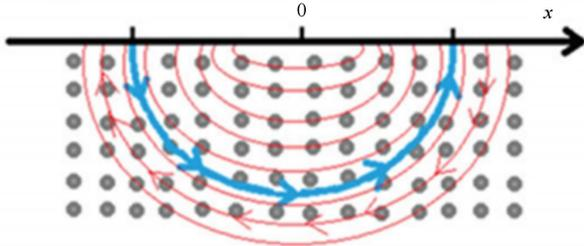
Fig. 12. (color online) Schematic view of the two-point 1<sup>st</sup> order MP on the shorting plate (red line: electric field, dark point: magnetic field, blue line: electron trajectory). From Ref. [7], Fig. 14.
