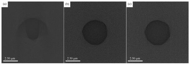
Fig. 3. A cross section of the gold particle reconstructed with (a) the raw projection images and projection image series corrected independently with (b) the GVB and (c) the MCM calibration procedures.
