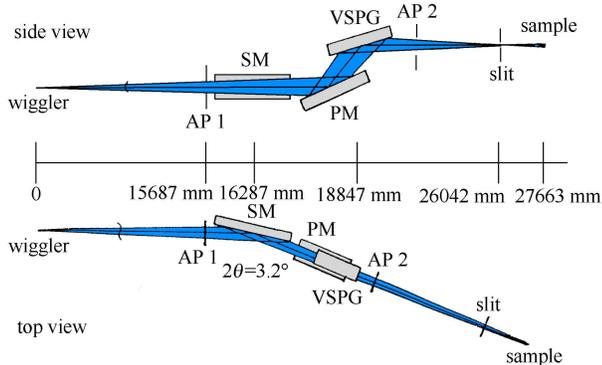
Fig. 1. Side view and top view of the beamline.
