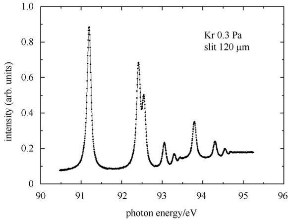
Fig. 3. The absorption spectrum of the krypton  $M_{4,5}$  edges.
