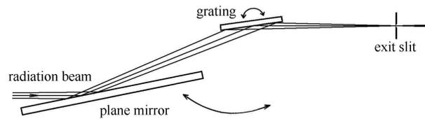
Fig. 2. The optical arrangement of the new monochromator.
