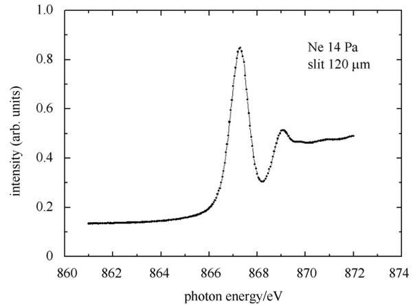
Fig. 5. The absorption spectrum of the neon K edge.
