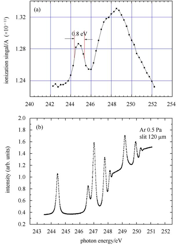
Fig. 4. The absorption spectra of the argon  $L_{2,3}$  edges before (a) and after the upgrade (b).
