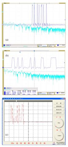
Fig. 10. (color online) Test for valid signal distinguishing. (a) The input signal #1 (all pulsed widths <3 ns, the sampling is not triggered);</li>
