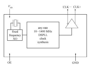
Fig. 4. The clock source circuit.
