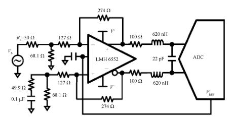
Fig. 3. The single-to-difference conversion circuit.
