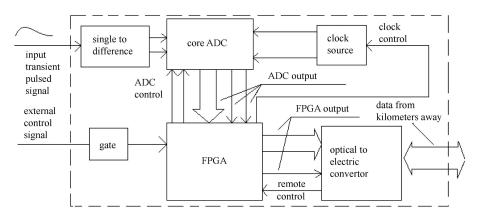
Fig. 2. The simplified measuring system circuit.
