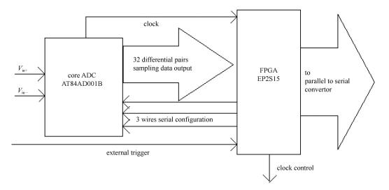
Fig. 5. The circuit with ADC and FPGA.
