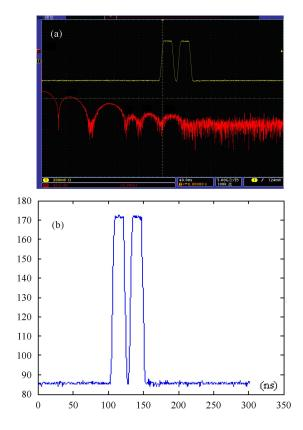
Fig. 7. Test for the automatic pretrigger. (a) Recording from the digital oscilloscope; (b) Recording from the digital transmission system.
