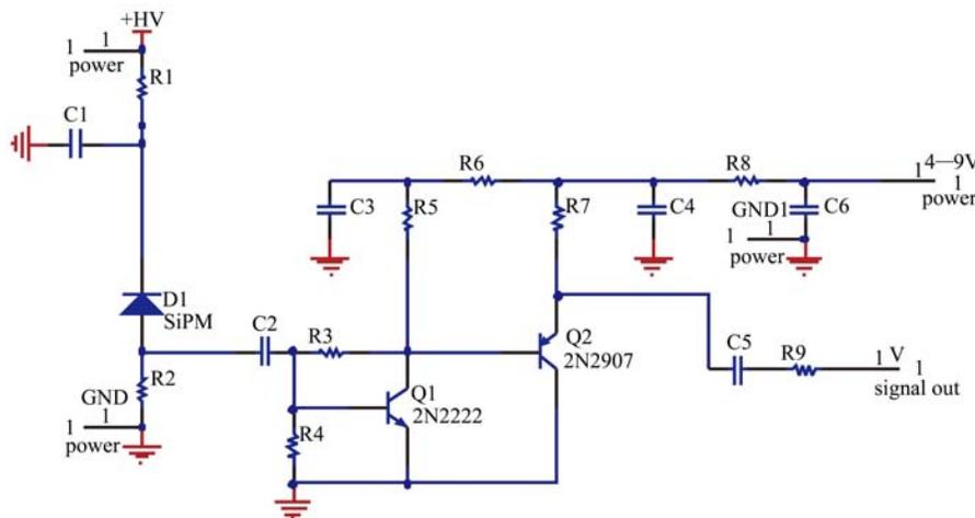
Fig. 1. The readout circuit connected to the SiPM.
