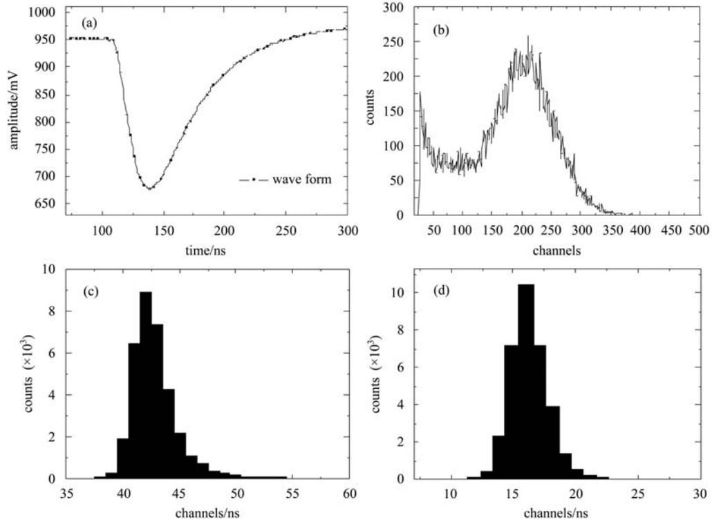
Fig. 2. (a) Typical signal waveform, (b) SiPM pulse height spectrum from the alpha spectrum by BC408, (c) the width of signal and (d) the width of the rise edge.
