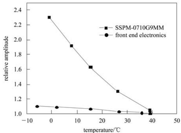
Fig. 6. The measured relative output amplitude as a function of temperature of SSPM-0710G9MM.
