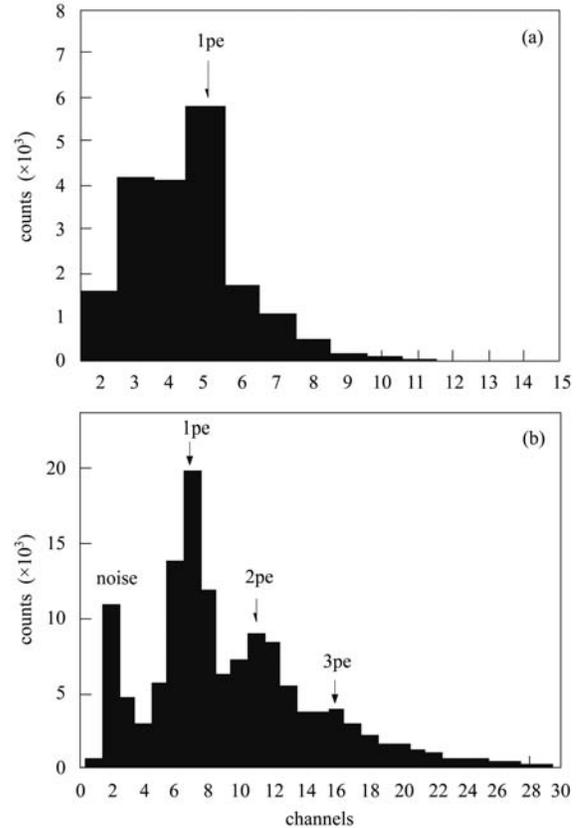
Fig. 3. MPPC S10362-33-025C dark count spectrum of  $V_{op} = 71.9$  V (Fig.(a)) and  $\Delta V = 2$  V (Fig.(b)).
