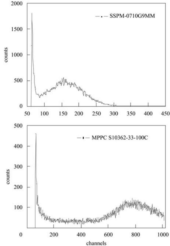
Fig. 5. The alpha spectrum tested at room temperature by BC408.
