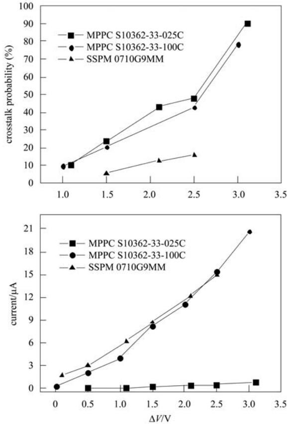
Fig. 4. The crosstalk probability and  $I$ - $V$  curve as a function of over-voltage ( $\Delta V$ ) at 26 °C.
