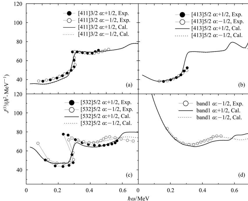
Fig. 2. Comparison between the experimental and calculated kinematic MOI  $J^{(1)}$  of the seven rotational bands in  $^{155}\text{Tb}$ . The experimental data are denoted by solid and open circles respectively. The calculated results for these bands are denoted by solid and dashed lines respectively.
