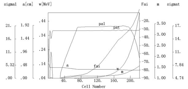
Fig. 1. The main dynamics parameters (signal is longitudinal phase advance, sigmat is transverse phase advance, Fai is synchronous phase, a is aperture radius, w is ion energy and m is modulation respectively).
