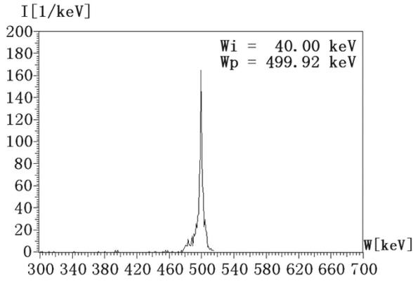
Fig. 2. Output beam energy spectrum.
