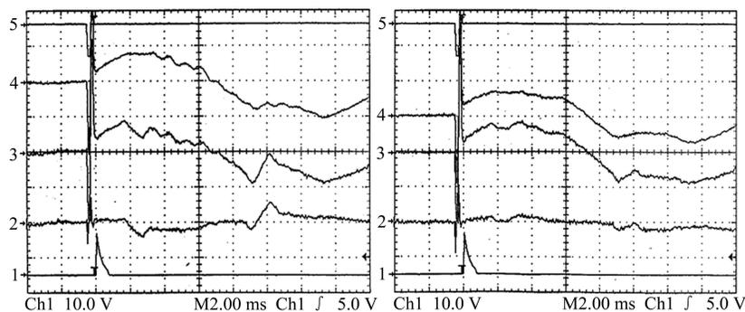
Fig. 4. The measured Y waveforms without (2 on the right) and with (2 on the left) steering magnets correction (1—triggering signal, 3—compound signal, 4—background signal, 5—pulse current in wire).
