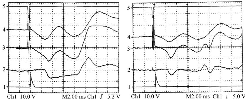
Fig. 2. The typical tilt (left) and offset (right) waveforms. The measured X waveforms (1—triggering signal, 2 on the left—net tilt signal, 2 on the right—net offset signal, 3—compound signal, 4—background signal, 5—pulse current in wire).
