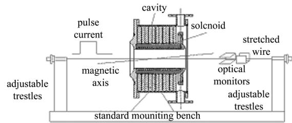
Fig. 1. The stretched wire technique.
