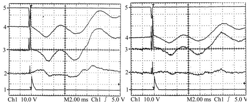
Fig. 3. The typical waveforms before (2 on the left) and after (2 on the right) adjusting the wire's position (1—triggering signal, 3—compound signal, 4—background signal, 5—pulse current in wire).
