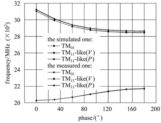
Fig. 8.  $\omega$ - $\beta$  diagram of simulation and measurement.
