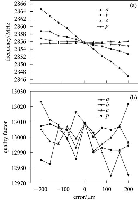
Fig. 5. (a) Relationship of  $TM_{11}$ -like ( $V$ ) mode:  $\partial f/\partial a=-14.78$  kHz/ $\mu\text{m}$ ,  $\partial f/\partial b=-46.24$  kHz/ $\mu\text{m}$ ,  $\partial f/\partial c=2.27$  kHz/ $\mu\text{m}$ ,  $\partial f/\partial p=-5.07$  kHz/ $\mu\text{m}$ ; (b) Quality factor vs. error of  $TM_{11}$ -like ( $V$ ) mode.
