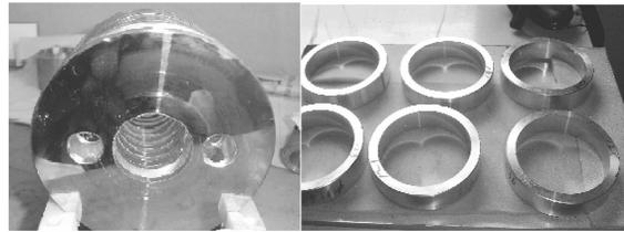
Fig. 2. The disks (left) and the cylindrical waveguides (right).
