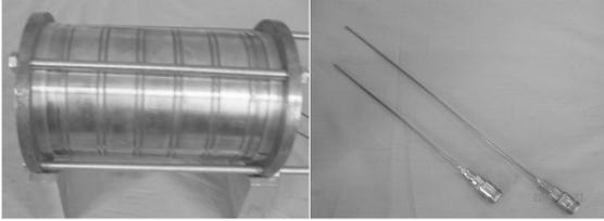
Fig. 7. The cavity prototype and the test coupling loops.
