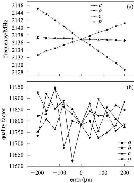
Fig. 4. (a) Relationship of  $TM_{010}$  mode:  $\partial f/\partial a=22$  kHz/ $\mu\text{m}$ ,  $\partial f/\partial b=-39$  kHz/ $\mu\text{m}$ ,  $\partial f/\partial c=-2.5$  kHz/ $\mu\text{m}$ ,  $\partial f/\partial p=-3.1$  kHz/ $\mu\text{m}$ ; (b) Quality factor vs. error of  $TM_{01}$  mode.
