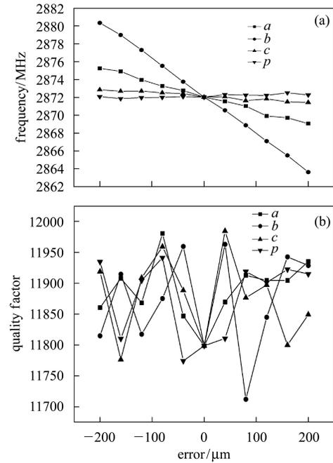
Fig. 6. (a) Relationship of  $TM_{11}$ -like ( $P$ ) mode:  $\partial f/\partial a=-21.09$  kHz/ $\mu\text{m}$ ,  $\partial f/\partial b=-42.56$  kHz/ $\mu\text{m}$ ,  $\partial f/\partial c=-2.49$  kHz/ $\mu\text{m}$ ,  $\partial f/\partial p=3.4$  kHz/ $\mu\text{m}$ ; (b) Quality factor vs.  $TM_{11}$ -like ( $P$ ) mode.
