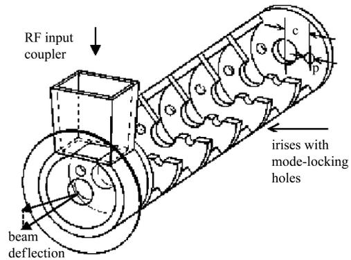
Fig. 1. The coupler and the suppressor's direction.
