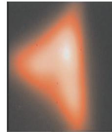
Fig. 4. Ion beam on a tantalum foil after extraction. Extracted ion current 5mA.
