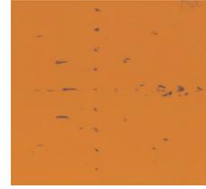
Fig. 2. Pepper pot figure of a  $\text{He}^+$ -beam behind the spectrometer.
