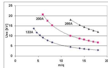
Fig. 9. Required extraction voltage for different  $m/q$  ratios. Three individual magnetic flux densities are shown.
