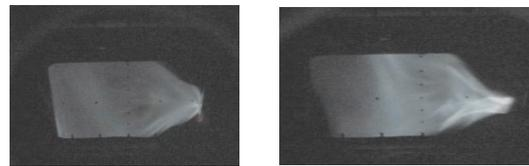
Fig. 8. Analyzed beam of one selected charge state on VT3. The screening voltage is set to zero in the left figure, and to  $-2$  kV in the right figure, respectively.
