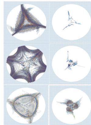
Fig. 11. Different cuts through the plasma chamber: injection side (top row), mid of plasma chamber (second row), extraction side (bottom row). The left column shows all trajectories, whereas the right column shows extracted ions only.
