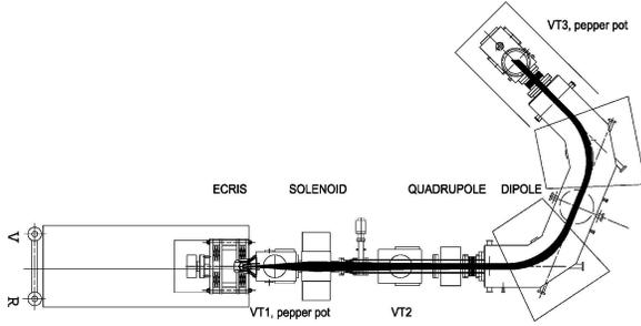
Fig. 1. EIS test bench with simulated 3D-beam envelope.
