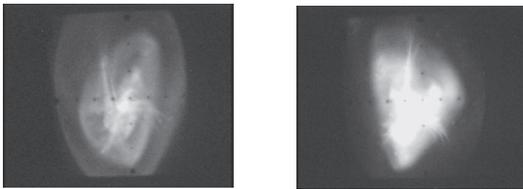
Fig. 5. Influence of gas pressure on the beam profile at the first VT1.
