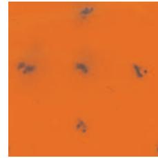
Fig. 3. Central part of the pepper pot figure of a  $\text{He}^+$ -beam behind extraction. Extracted ion current 5mA.
