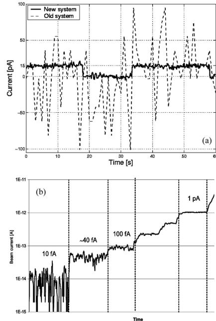
Fig. 3. The improvement of the beam intensity measurement system. The upper picture shows the noise of original configuration (with Keithley picoammeter) and the measured ion beam intensity with the first “homemade” system. The lower picture shows the measurement using the present measurement configuration.
