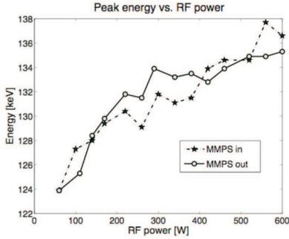
Fig. 1. The intensity distribution peak as a function of microwave power.
