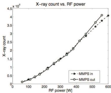
Fig. 2. Total X-ray count as a function of microwave power.
