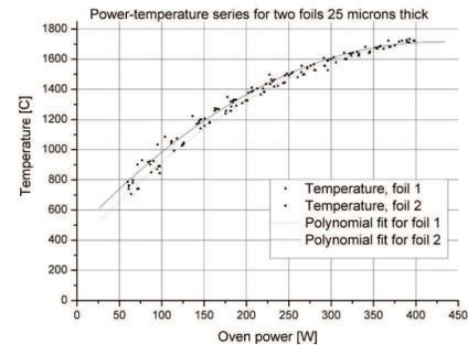
Fig. 6. Temperature of oven as a function of power.
