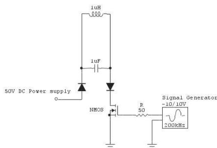
Fig. 4. Resonant circuit of the inductively heated oven.
