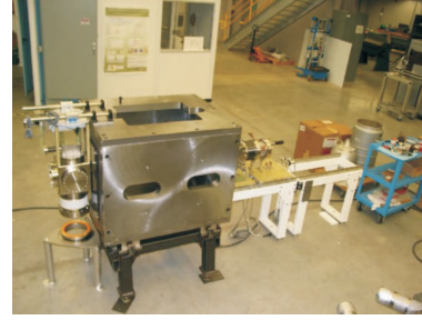
Fig. 4. The SuSI magnet yoke with the injection and extraction hardware and plasma chamber with electrical isolation ready for tests, on September 12, 2006.
