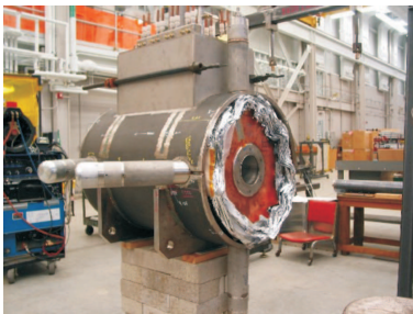
Fig. 3. The SuSI magnet cryostat before the super insulation is applied to the front and back end of the liquid nitrogen thermal shield on September 12, 2006.
