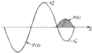
Fig. 1. Longitudinal wake-potential of a symmetric charge bunch.
