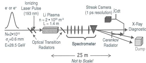
Fig. 3. Experimental layout of the laser-plasma acceleration experiments at the SLAC FFTB.
