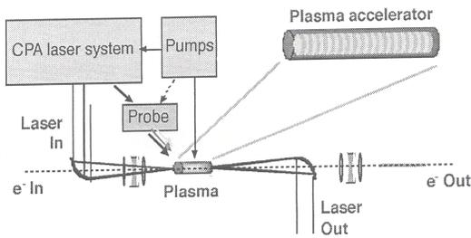
Fig. 4. Schematic layout of a laser-plasma acceleration laboratory.
