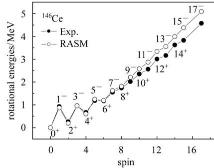
Fig. 5. Theoretical (open circle) and experimental (solid circle) energies of the octupole deformed bands of the  $^{146}\text{Ce}$  nucleus as a function of spin.
