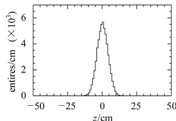
Fig. 1. The distribution of IP in the  $z$  direction measured with  $\psi(2S) \rightarrow \text{hadrons}$  at BES II.
